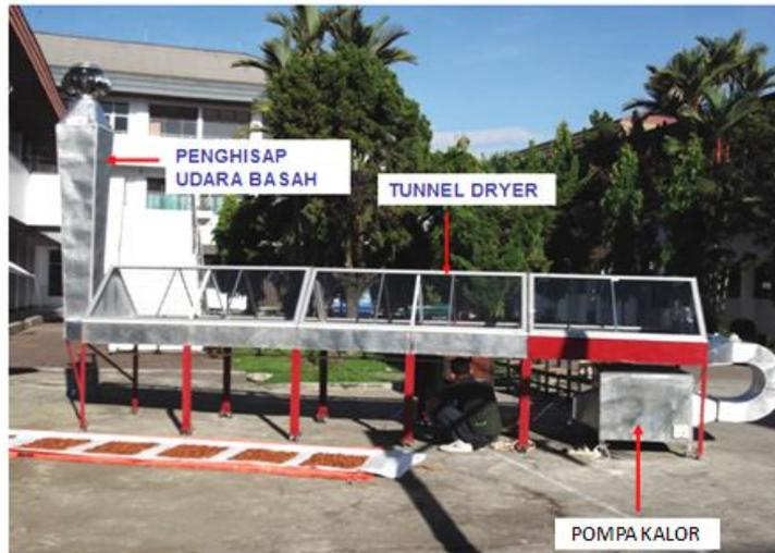
Gambar 1: Photo Alat pengering lorong berbantuan pompa kalor
